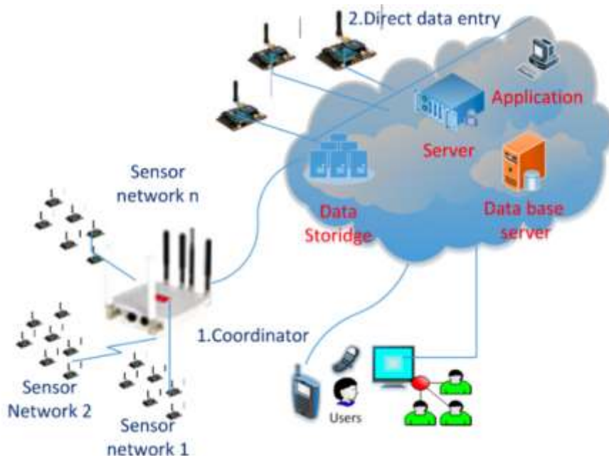
Figure 16: Sensor network with a cloud structure
